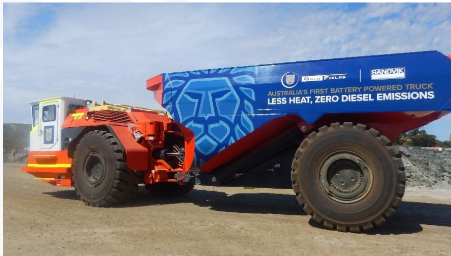
St Ives Sandvik 50T Battery Electric Underground Truck
