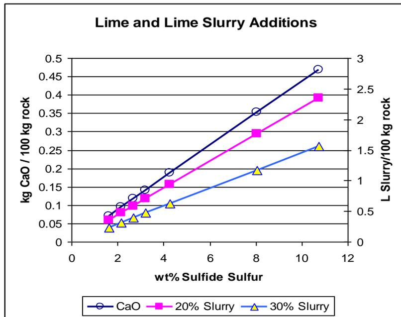
$$y=0.437(\text{wt}\%S) \text{ L slurry}/100\text{kg Rock}$$
